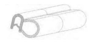
Sealing profiles as a combination between PVC edge trim and sponge rubber can have up to two glued joints.
